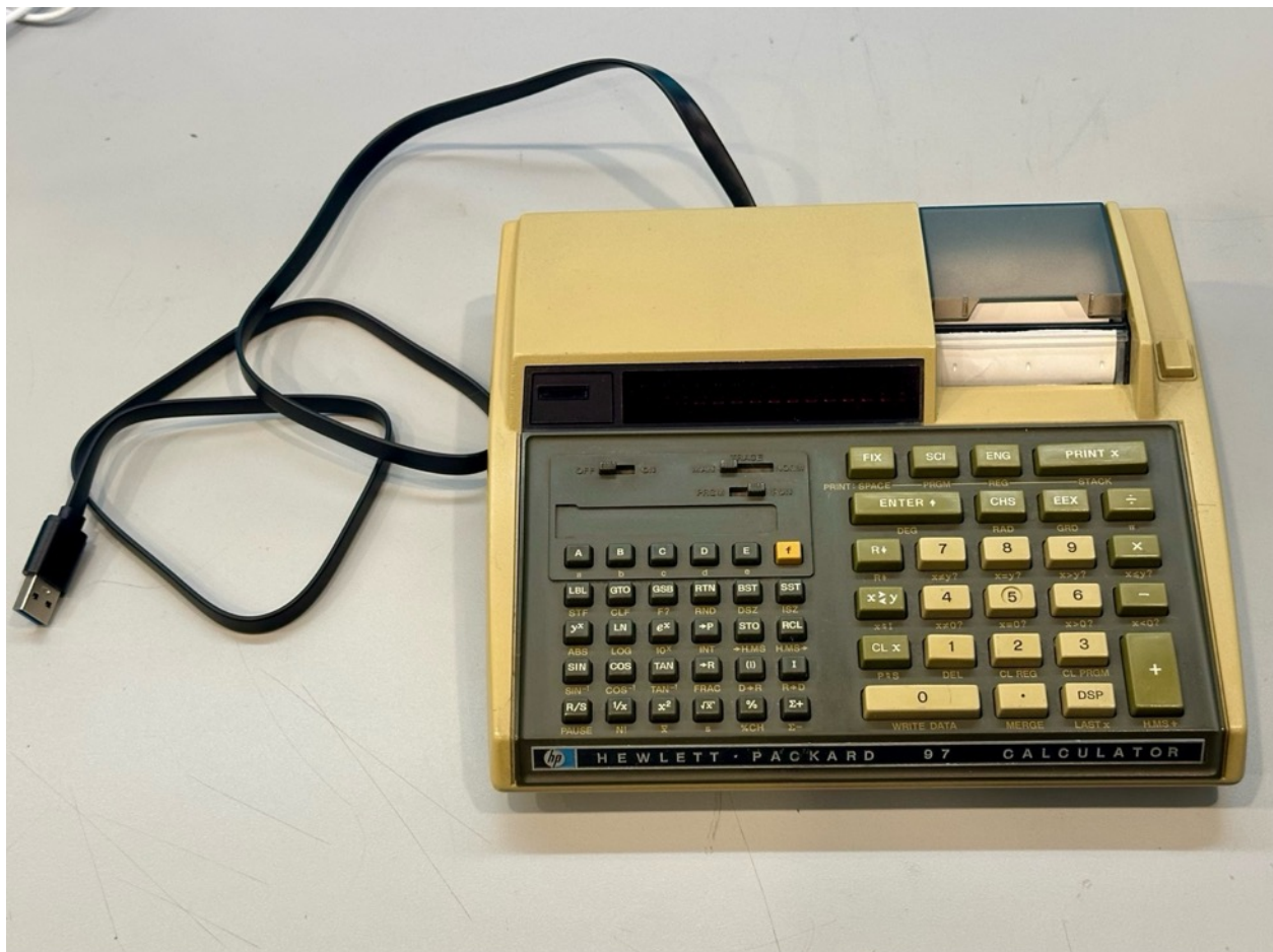
Figure 1: The final result... an HP97 with a flat USB-A cable coming out of it (I used a 3-foot cable) that does not need (and should not have installed) the original NiCd battery pack and will work well on less than 2W of 5V USB power. This should last until 2125, or so. ☺
