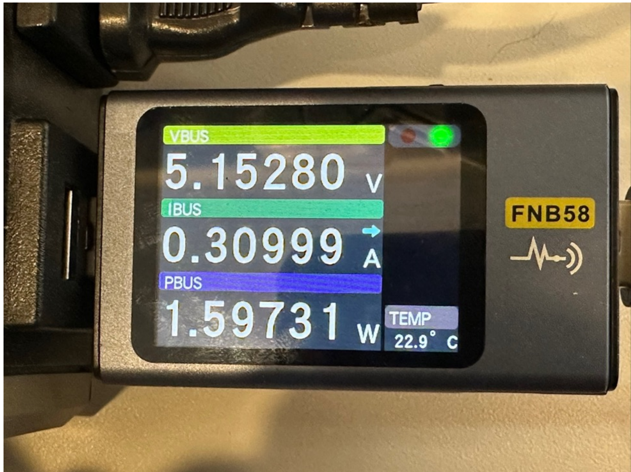
Figure 3: Current draw is around 310mA with all display segments on. Not much different, still less than 400mA, when printing. This does not show peak currents, but my opinion is that it works. Implement at your own risk but if you do, enjoy. ☺
